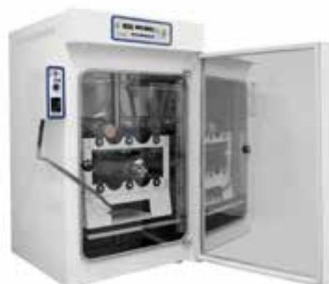
Four Dia.100-120mm roller bottles can be installed with speed controller on the outside
