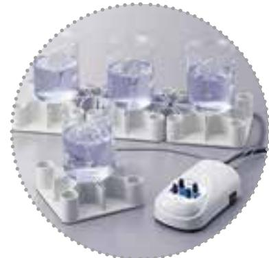
Different speed for connected stirrers
