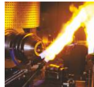
AUTOMATIC JOINT FORMING MACHINE : 2000 pcs per shift
