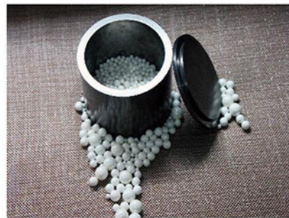
Hard Alloy mill pot can be matched with zirconia balls
