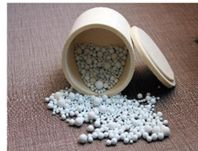
Corundum mill pot can be matched with alumina balls
