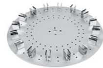
Cat. No.: 18900161 Type 2 plate 16*15ml centrifuge tube
